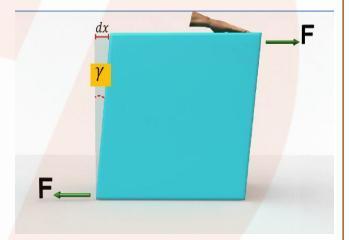
The SI unit of shear modulus is N/m<sup>2</sup>
