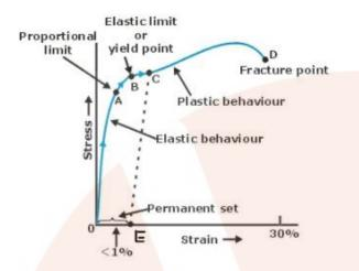
Figure shows the stress-strain curve for a metal wire which is gradually being loaded.
