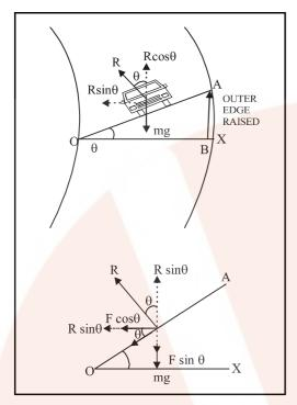
Three forces are acting on the vehicle as shown in Fig.
